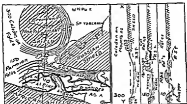
FIGURE 55—The build of Europe determined by the squeezing of weak sediments to make Young Mountains between the three Shields. At the right are given three vertical sections (along the line XY) at the dates specified. Figures represent millions of years ago. R.S. Russian Shield.
